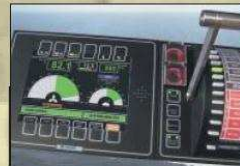
Propulsion Control System
